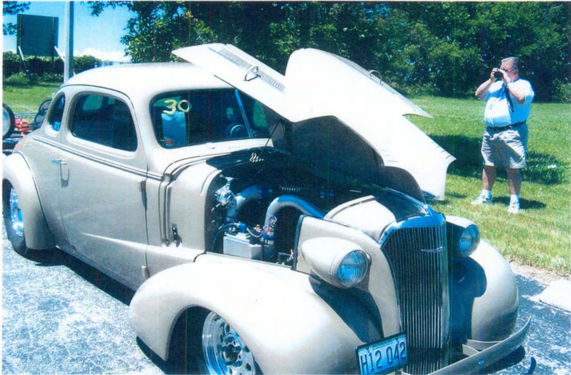
This turbo charged 292" Chev really fills the underhood area of a 37 Chev. Huge turbo blows through an intercooler into three Holley 2BBLs.
