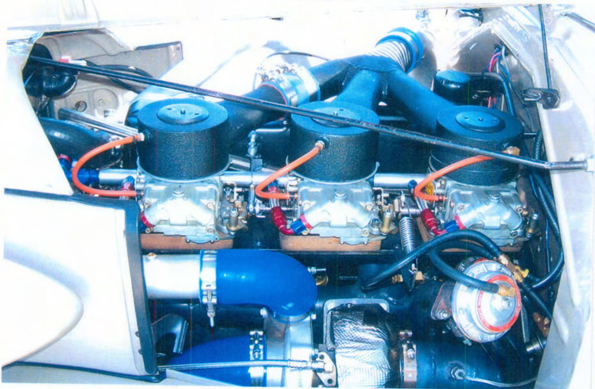
This turbo charged 292" Chev really fills the underhood area of a 37 Chev. Huge turbo blows through an intercooler into three Holley 2BBLs.
