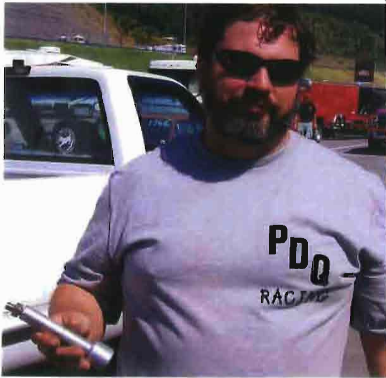
Dan Gravatt, Phil Stonbeck's brother in law, drove Lou Madsen's 64 Dart with the 5 speed transmission at Bristol. Vigorous shifting resulted in this broken shifter handle.
